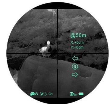
orientation between X-axis (left-right) and Y-axis (up-down) while the moving distance is displayed synchronously above the icon.
